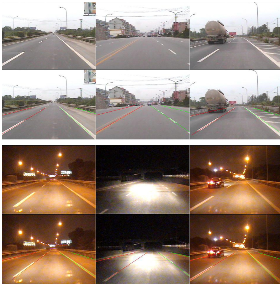
Fig. 5. Lane detection at daytime and night. First row: input images, second row: detection results.
