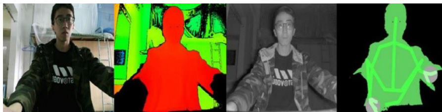
Fig. 6. RGB image, depth image, near-infrared image, and skeleton captured by Kinect.
