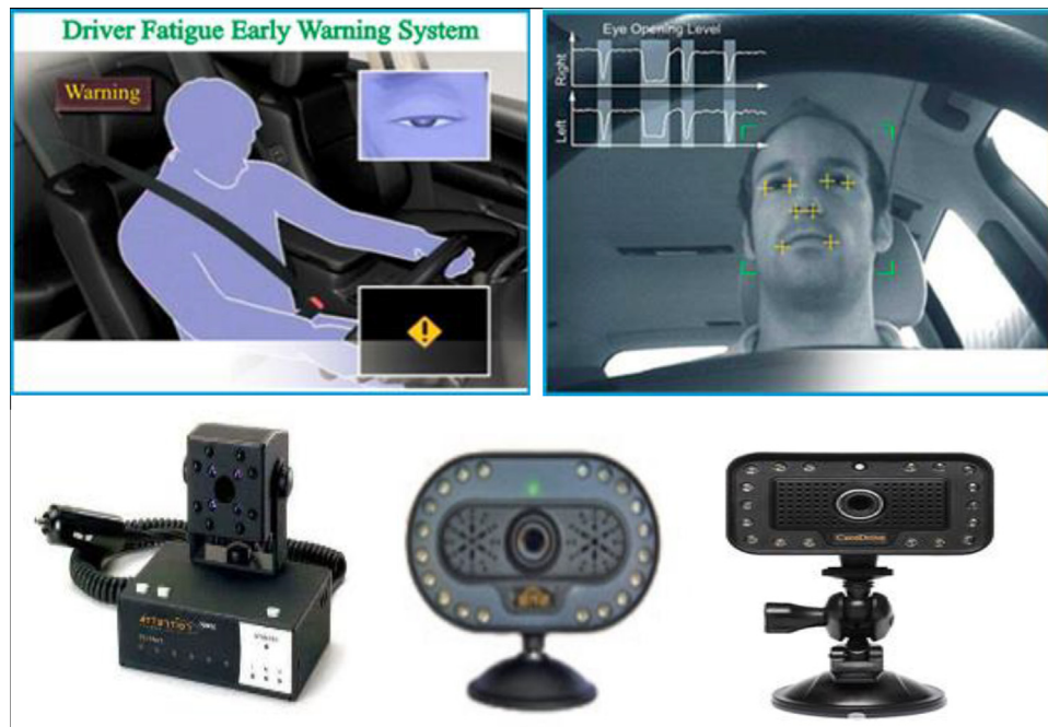
Fig. 2. Different fatigue detection products based on driver behavior features (DD850, gogo850, and MR688). Source: Images extracted from Nanjing Yuanqu Technology Co., Ltd. (2020).
